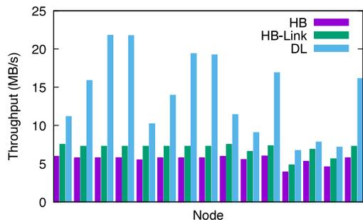
**Figure 15:** Throughput of each server running different protocols on the Vultr testbed. HB stands for HoneyBadger, HB-Link stands for HoneyBadger with inter-node linking, New stands for DispersedLedger.
