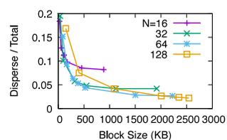
**Figure 13:** Fraction of dispersal traffic versus total traffic at different scale and block size.
