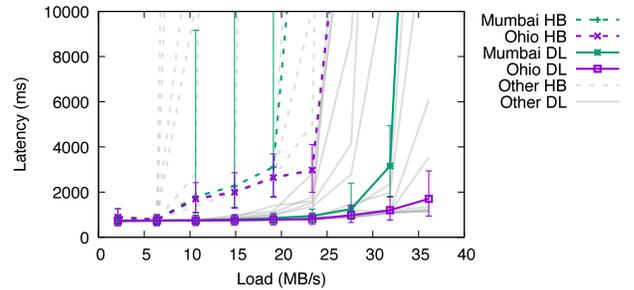
**Figure 10:** The median latency of DispersedLedger (solid) and HoneyBadger (dash) under different offered load. Error bar shows the 5-th and the 95-th percentiles. Two locations with good (Ohio) and limited (Mumbai) internet connection are highlighted.
